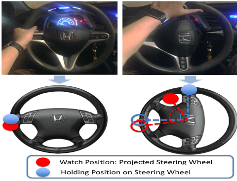
Fig. 7: Holding position and the projected position of smart watch on steering wheel.
